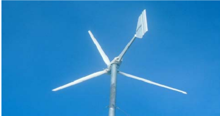
Figure 7. The Westwind 10 kW horizontal wind turbine. From [9]
